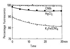
Percentage relative fluorescence readings of thiochrome from eluates of the loaded tea infusion (1 g/50 ml) kept at 85 °C for various times. Here 1.25 ml of the infusion was loaded on to the Decalso column and 5 ml of the eluate was used for assay by the 3 reagents. If only 0.25 ml of the brew was used for column loading all 3 assays yielded the CNBr curve.
